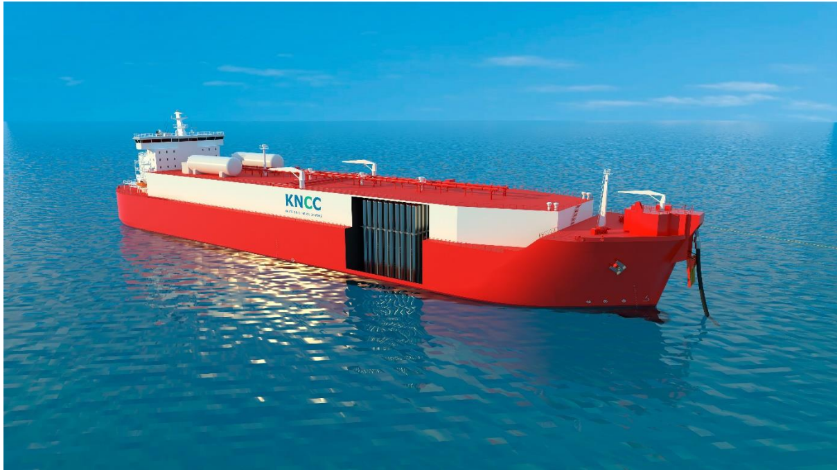
Image of liquefied CO 2 carrier utilising the innovative LCO 2 -EP technology and offshore bow offloading system
