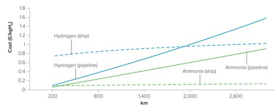
Note: Hydrogen transported via pipeline is gaseous and liquefied for shipping. Costs include both the transport and storage required; not the conversion, distribution or reconversion.
