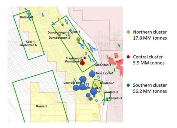
Figure 6 shows how the leads and structures within each of the clusters are situated in relation to a hypothetical series of three CCS project developments, with a development radius of 15 km from three central development locations.
