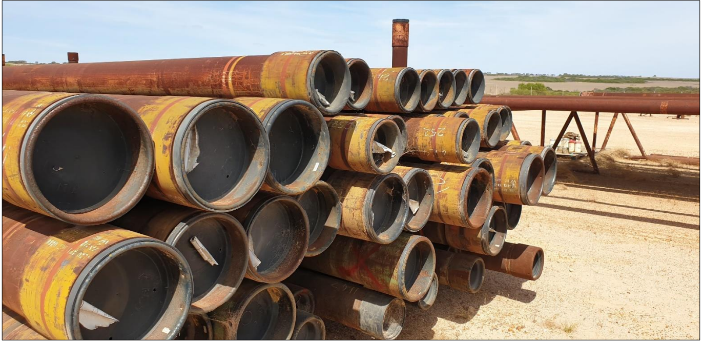
KPS secured 9 5/8" and 7" casing joints
