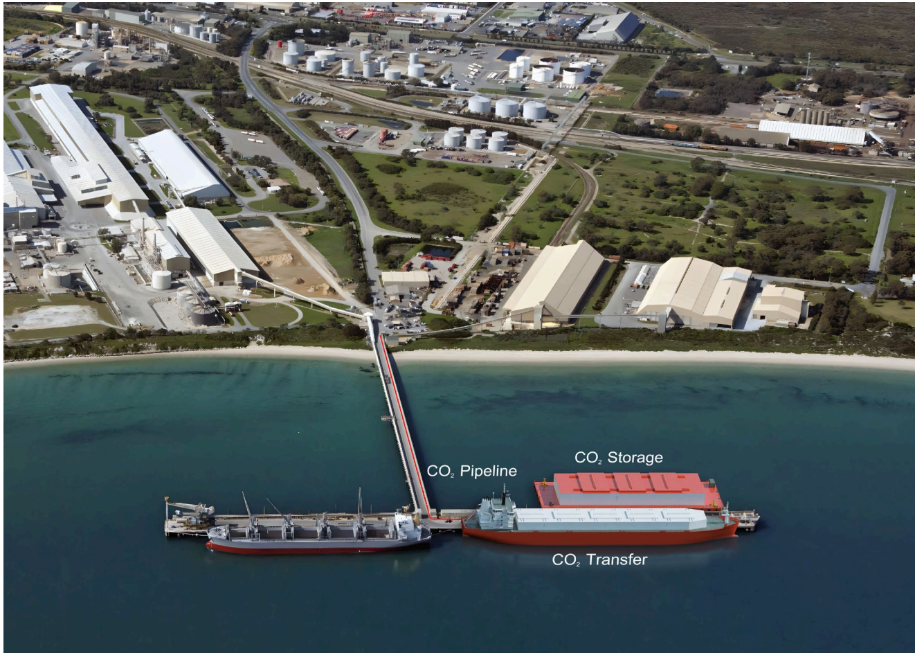
Concept 1 - CO 2 Export Terminal, offshore barge storage utilizing existing jetty facilities
